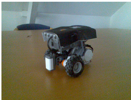
Figure 5.2: The robot that serves as agent and follows the line on the floor in the environment.
