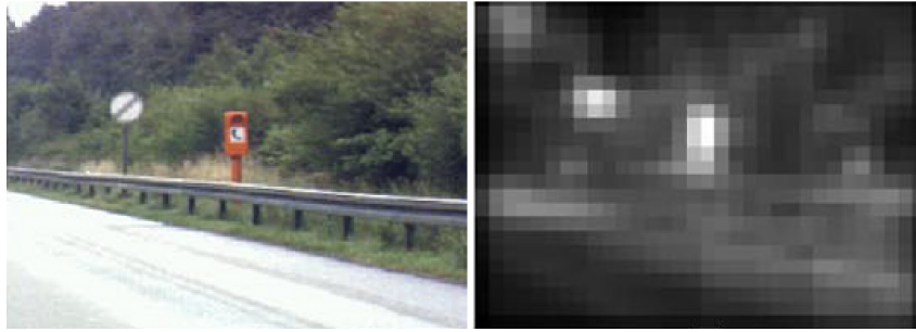
Figure 2.6: A saliency map computed with the visual attention system of Itti et al. [28] with the corresponding input image on the left. (Taken from [28])
