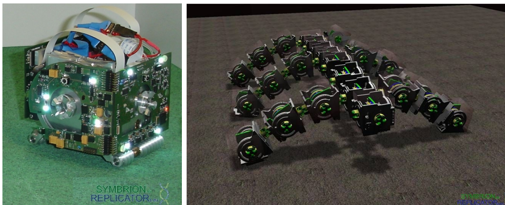
Figure 1.1: Left: REPLICATOR robot prototype, courtesy of Replicator and Symbrion consortia. The robots have autonomous screw drives and four connectors to connect to other modules. There are also four cameras mounted on each side to detect the state of other robots. Right: Motivating example. 23 REPLICATOR modules can assemble to a hexapod on the plane. The structure can then stand up and walk using internal hinge joints. This thesis focus on graph grammar-based, stochastic algorithms to enable self-assembly of such a structure from limited number of blocks.
